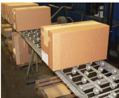
Skate-wheel conveyors can be easily set up wherever needed and work well for light loads.
