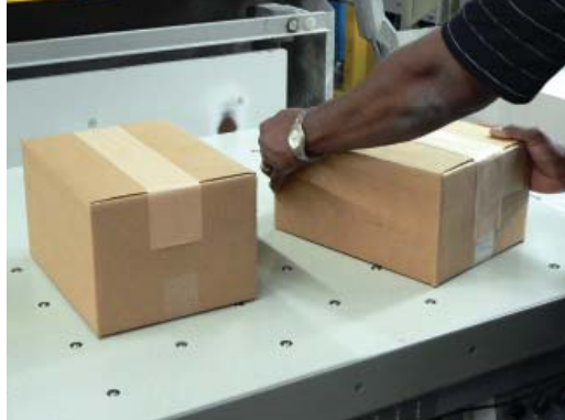
An airball table makes it easier to slide containers, thereby reducing workers' efforts.
