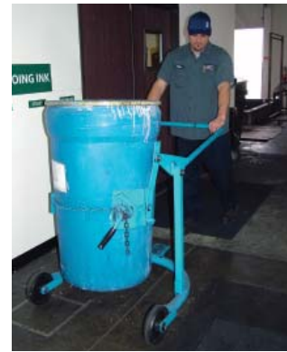
This drum dolly lifts and transports drums.
