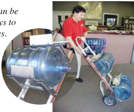
Two-wheel hand trucks work well for transporting bottles or cylinders over short distances.
