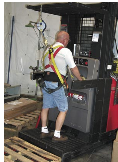
The operator of an order picker type forklift must wear a safety harness to protect against the fall hazard at an elevated location.
