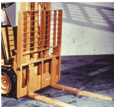
A backrest extension keeps the load from falling rearward.
