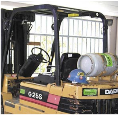
An overhead guard can deflect objects falling from above.
