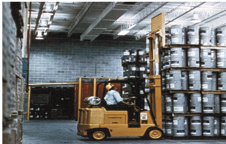
Internal combustion engine forklifts can cause carbon monoxide poisoning when used indoors if the engine is not kept tuned and the area well ventilated.
