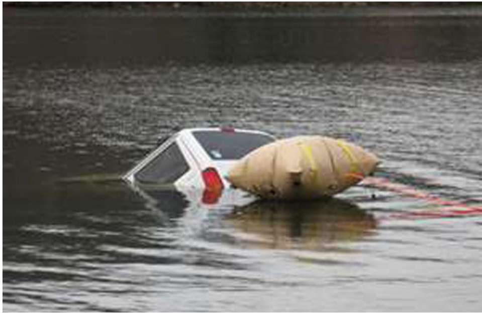
Recovery of vehicle—Staying clear of load
