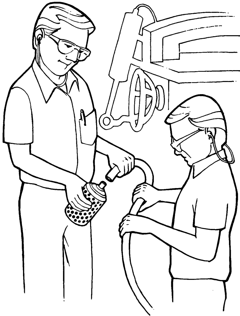
Many common noise problems, such as air exhaust noise, are simple to control with commercially available mufflers.
