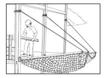
• The nets must be as close as practicable under the working surface, but never more than 30 feet below;
