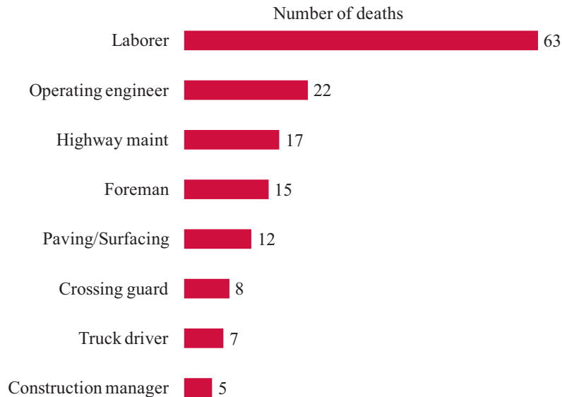
46e. Fatalities involving vehicles and heavy equipment at road construction sites, selected occupations in construction, 2008-2010 total
